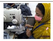
NC Photo-1: Eye guard of Bartack was found in displaced condition
