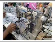
NC Photo-2: Eye guard of flatlock machine was found in displaced condition
